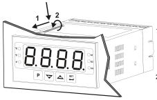
This unit is designed for panel mounting.
