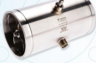
Designed specifically for harsh environments, the TMS0600 meter provides durability and longevity in abrasive and slurry applications to deliver accurate, reliable results. This meter has a flow range from 200 to 2,900 GPM, provides +/- .5% standard accuracy, and is repeatable to +/- 0.10% over the entire flow range. The TMS0600 features stainless steel construction and Victaulic® end connections.
