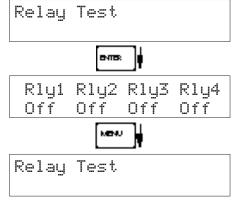
Press Enter to test the relays.
