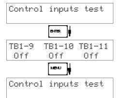
Press Enter to test the control inputs.
