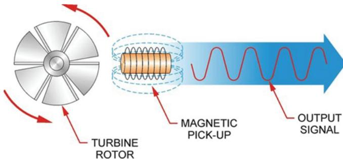
Figure 1: Electric signal generated by rotor movement
