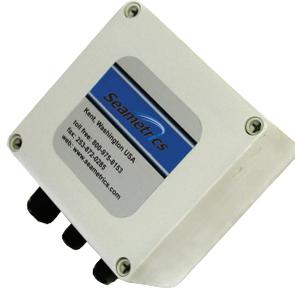
The housing is rugged molded ABS plastic, NEMA 4X rated. It can be wall or panel mounted. The PC42 can be hardwired to the AC main supply or plugged into a standard outlet using the included power cord. Inside there are separate terminals to connect the two devices to the fully isolated supplies.
