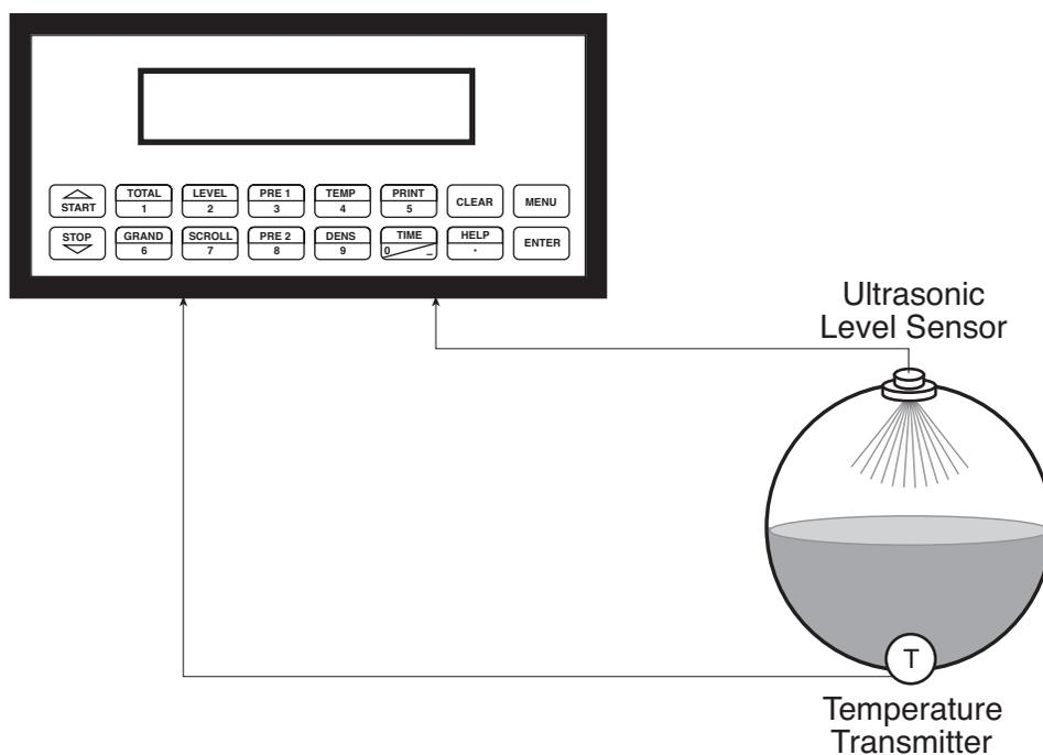
**Batching Volume, Corrected Volume or Mass from Tank Level**
