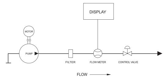
Install the meter upstream from control valves and fluid regulators if possible. Back pressure from control valving is beneficial for stable running.
