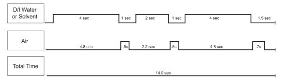
At the end of a shift or overnight, leave cleaning solvent or DI water with appropriate cutting agent in the meter, under pressure, to soak. This helps keep unflushed residual paint from drying and helps subsequent startups. Opening a meter after a flush cycle will help determine if the meter is being cleaned thoroughly by the purge.
