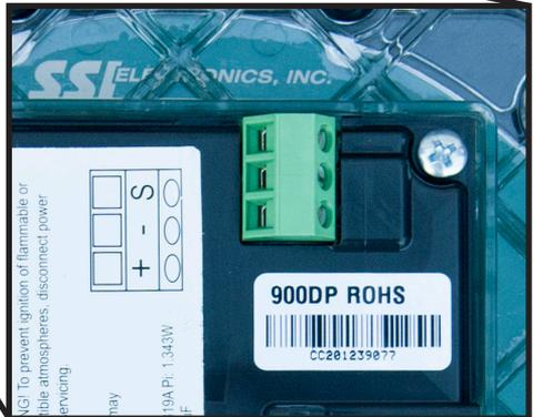
Auxiliary power and pulser connection at meter. Note three connections: DC+, DC-, and Pulser Signal.
