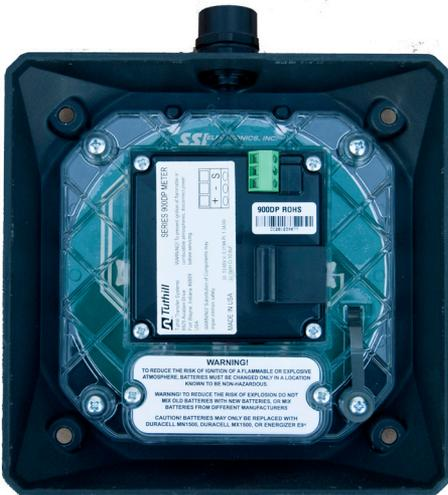
900CDP Battery and Wiring Access
