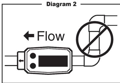
Upstream from the turbine, allow a minimum straight pipe length at least 10 times the internal diameter of the turbine. For example, with the 1 inch turbine, there should be 10 inches (25.4 cm) of straight pipe immediately upstream. The desired upstream straight pipe length is 20 inches (50.8 cm).
