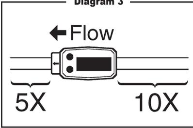
A typical back pressure of 5 to 50 PSI (0.34 to 3.4 bar) will prevent cavitation. Create back pressure by installing a control valve on the downstream side of the meter at the proper distance detailed above.
