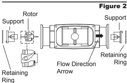
2. Using a small tool such as a screwdriver or awl, gently pry one retaining ring from its groove. Remove the support. If necessary, use needle nose pliers. Little or no force should be required.
