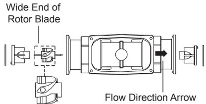
8. Turn the turbine over and drop the second turbine support into place. Put the final retaining ring into position.
