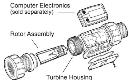
2. Use your fingers to gently remove the rotor assembly from the groove. Do not use force to remove the rotor assembly.
