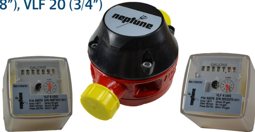
Red Seal Measurement VLF (very low flow) flowmeters have been designed to measure the flow of light fuel or diesel oil. They are available in three different sizes: 1/8" (VLF 4), 3/8" (VLF 8), and 3/4" (VLF 20) to measure flow rates ranging from 0.25 to 390 gph. The oscillating piston of these flowmeters forms two measuring chambers that are alternately filled and emptied. The passing oil is measured by fractions reflected by the register.
