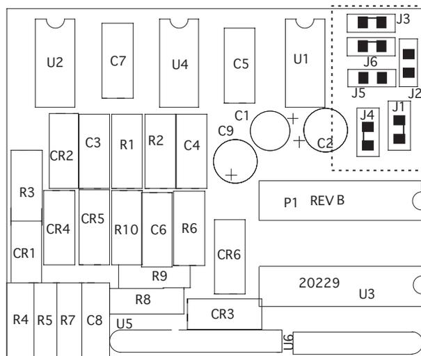
If the unit has the millivolt input bd.# 20229, The A inputs can be solder jumper programmed to accept either a low millivolt or 4-30 V input. The B input should always be set for 4-30 V. Each unit shipped is programmed according to part number. If solder jumpers are made, the part number should be modified to reflect the changes made
