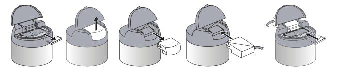
Do not hold the center of the retaining clip when inserting or removing it. Hold both ends and slowly insert or remove it. Ensure that that the lugs on the clip ends are pointed upward. Ensure the optical port is not blocked by foreign substances.
