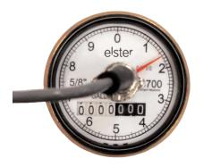
HSP (High Speed Pulse) adds a high frequency output capability to bronze body C700 meters while retaining the direct read register readability. The unit is a Missouri style register can that can retrofit direct read meters using appropriate retaining ring and housing combinations. The sensing element is a hall effect magnetic switch providing a 50/50 switch ratio.
